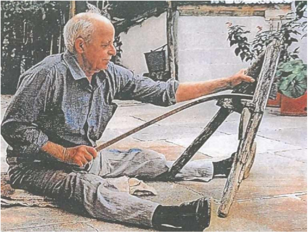
Bending the rib of the frame.
